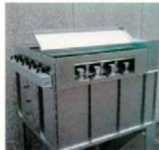
The roof consists of sectioned loose panels only requiring a height to the ceiling of 500 mm. The panels are designed to ensure the highest possible density.
